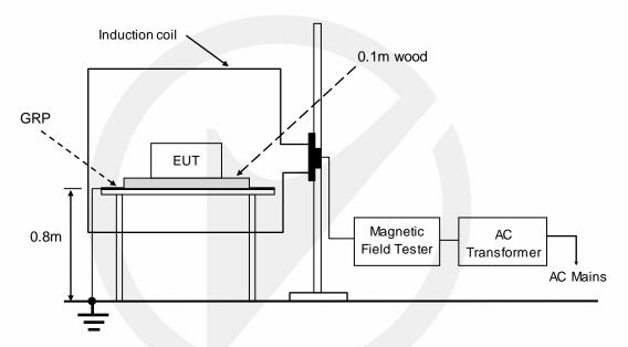
GRP: Ground reference plane EUT: Equipment under test
