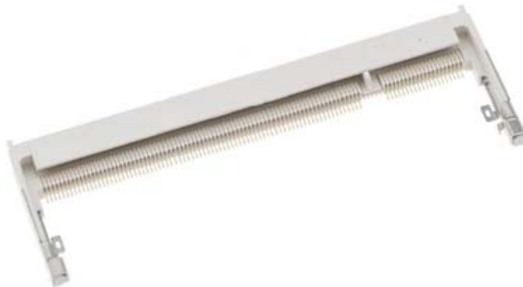
Figure 2. SODIMM Socket (2.5V, H=5.2mm, on the baseboard)
